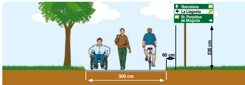
Figure 43. Location of direction traffic signs
