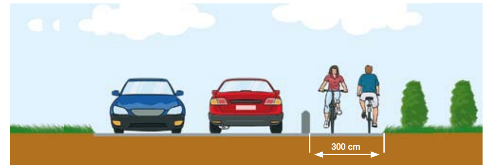
Figure 4. Protected two-way cycle lane in an interurban area
